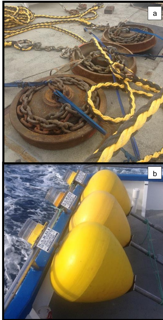
Figure 2. Mooring configurations (a) and navigation marker buoys (b) used to anchor the acoustic receivers in the Neptune Islands Group during 2015–16.
