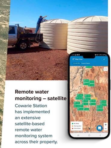
Water level sensors and rain gauges were installed at various locations across the property. The water level sensors are used to monitor tank levels, enabling real-time reporting on water trends, consumption and alerts. Following big rain events, these sites are inaccessible, preventing direct assessment of rainfall levels. Rain gauges are able to be checked remotely to capture accurate rainfall records across the property.
