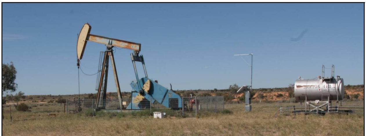
Fig. 46. A production well: the “nodding donkey” pump, and hydrocarbon storage tank.
