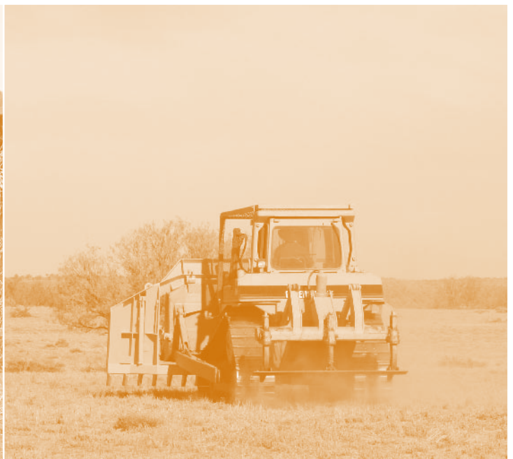
D6 Dozer with stick rake and blade plough attachment to remove dense infestations and large athel pine trees
