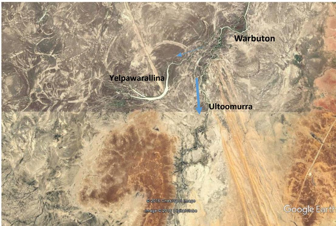
**Figure 14. Flow distribution in the upper Warburton in May 2016 near the peak of the first 2016 regional flow peak in the Warburton. Only 3% of the Warburton flow entered the Yelpawarallina channel. Larger flood events results in floodplain flow into Yelpawarallina too.**
