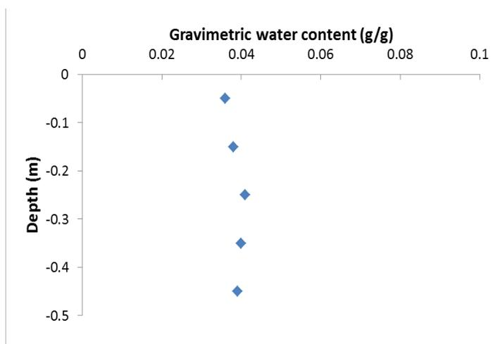
**Figure 28. Mean gravimetric soil water conditions from 51 soil profiles collected in May 2014.**
