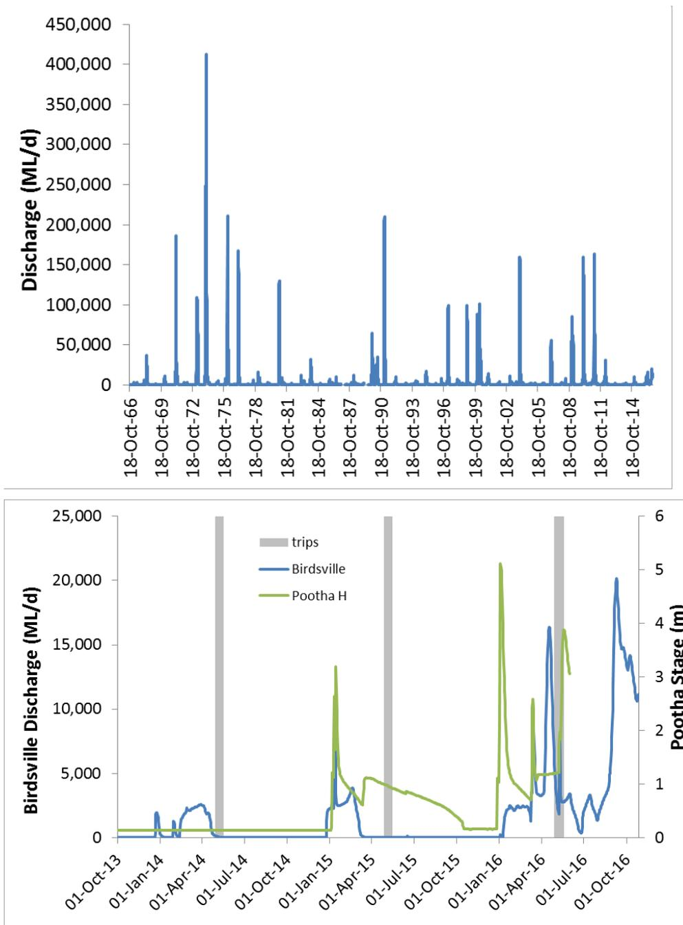
**Figure 1. Hydrograph of Birdsville gauging station record for Diamantina River for the period 1966-2016 (top panel). The lower panel shows the Birdsville discharge hydrograph (blue) and the Poothapoota (Warburton River) stage hydrograph (green) for the flood years of 2014 – 2016. The periods of Diamantina River fieldwork are shown by the grey columns.**
