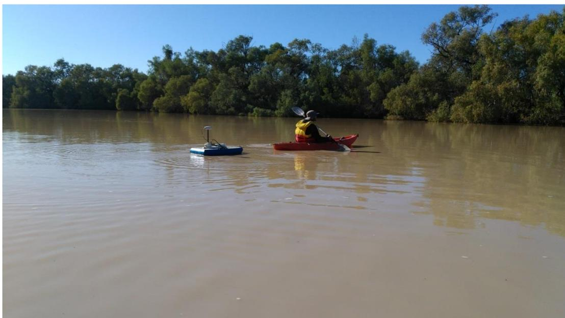
**Figure 4. Flow gauging using the ADCP at the outflow channels of Andrewilla Waterhole.**
