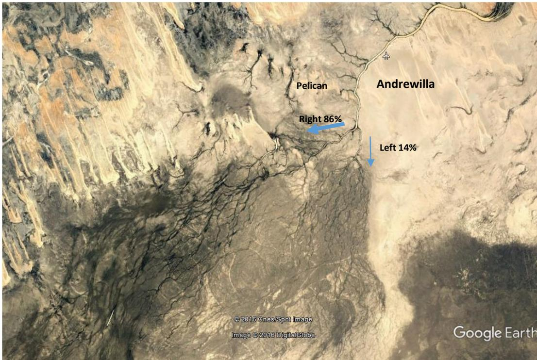
**Figure 12. Flow distribution downstream of Andrewilla Waterhole shown for May 2016. The left flow path feeds a poorly developed channel network and the right distributary feeds the main flow path towards Goyder Lagoon Waterhole.**
