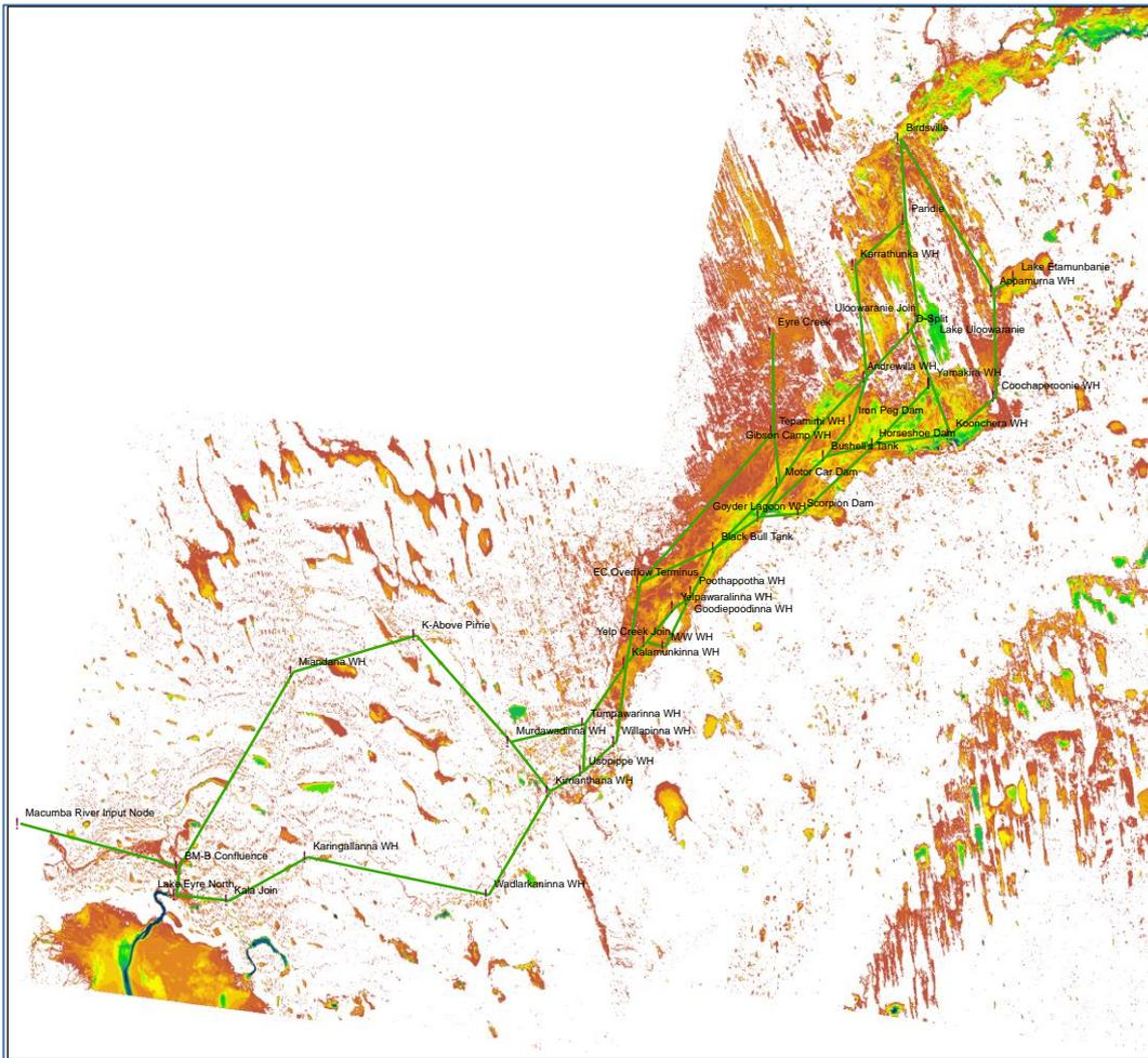
**Figure 15. Link-node network for the Source model of the SA Diamantina reaches (Osti 2015) superimposed on Geoscience Australia's Water Observations from Space (WOfS) frequency of inundation map.**
