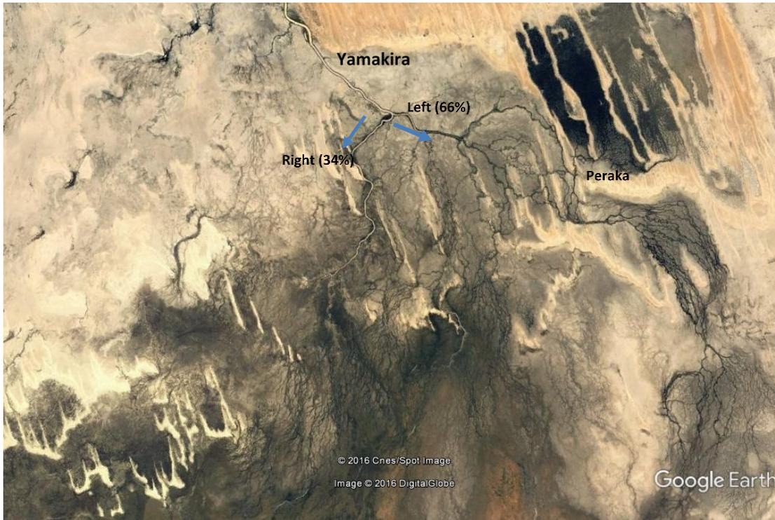
**Figure 11. Flow distribution downstream of Yammakira Waterhole shown for May 2016. The left flow path feeds Bobbiemoonga and Koonchera Waterholes and the right distributary feeds into a dense area of vegetation.**
