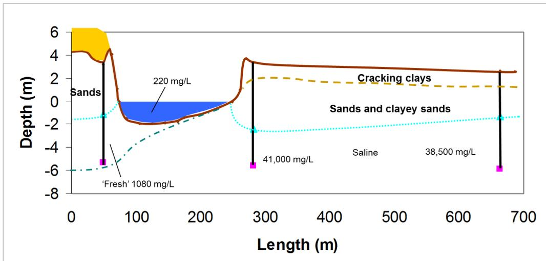
**Figure 19. Cross-section through Yelprawaralinna Waterhole showing groundwater characteristics and typical water level and surface water salinity during 2004-2006.**
