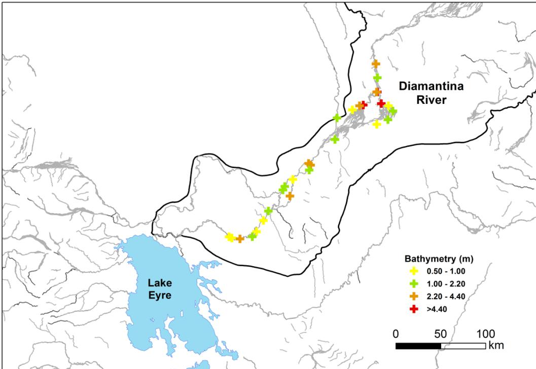
**Figure 7. Distribution of waterbodies on Diamantina River with bathymetric measurements collected during 2014-2016. The legend shows the ranges for the observed maximum cease-to-flow depth. One year's evaporative loss (assuming no inflow) is approximately 2.2 m.**
