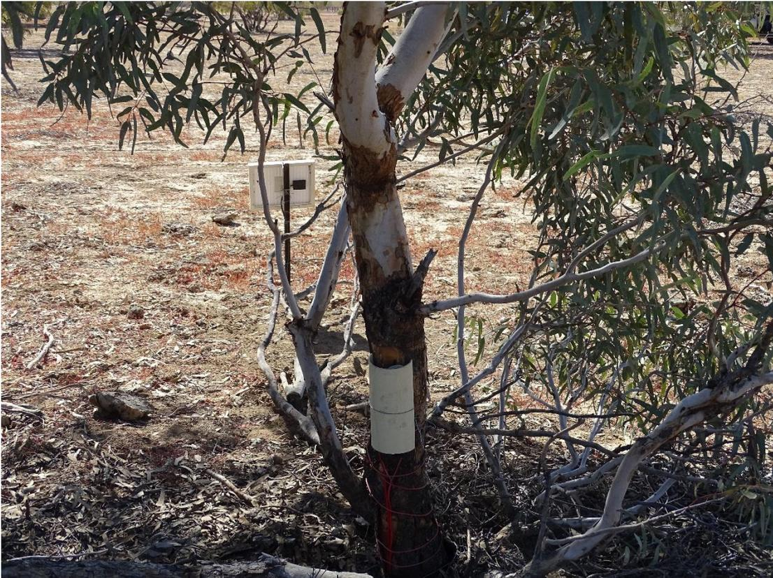
**Figure 6. Sap flow logger (covered by a half piece of PVC pipe to provide protection from animals) installed into a coolibah on the floodplain at the Double Bluff site. The sap flow logger only records from one stem and the whole of tree response requires that the circumferences of all stems are measured for the instrumented tree.**
