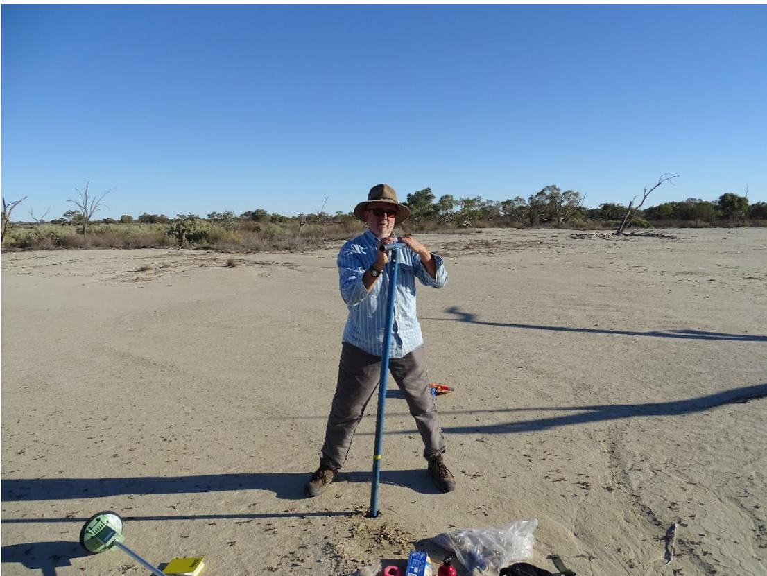
**Figure 5. Graeme Tomlinson collecting soil profile samples using an auger in an area without any nearby coolibah trees (see dead trees around the edge of this scalded high floodplain area). The differential GPS unit used to record location and elevation is lying on the ground in the left foreground. Cliff Camp floodplain, May 2015.**
