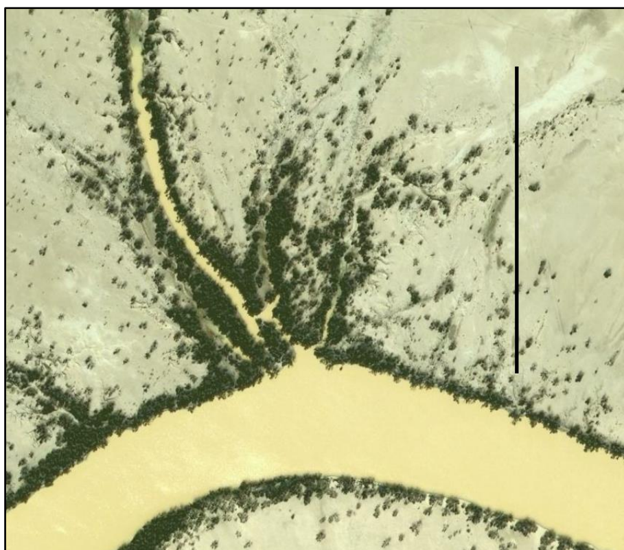
Fig. 46 A complex offtake at an Andrewilla distributary channel.
