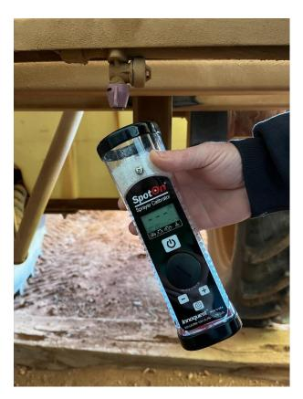
meter can be removed from under the nozzle. The screen will display the flow rate in litres per minute.
