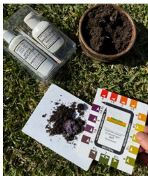
Use colour wheel to match colour and determine pH of soil sample.
