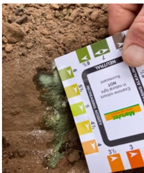
Use colour wheel to match colour and determine pH of soil sample.
