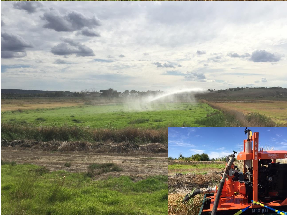
Figure 2-4(top) travelling irrigator in operation, and (bottom left) photograph showing full irrigation bay width was watered and (bottom inset) 4" diesel pump used to provide water to irrigator (via layflat hose)
