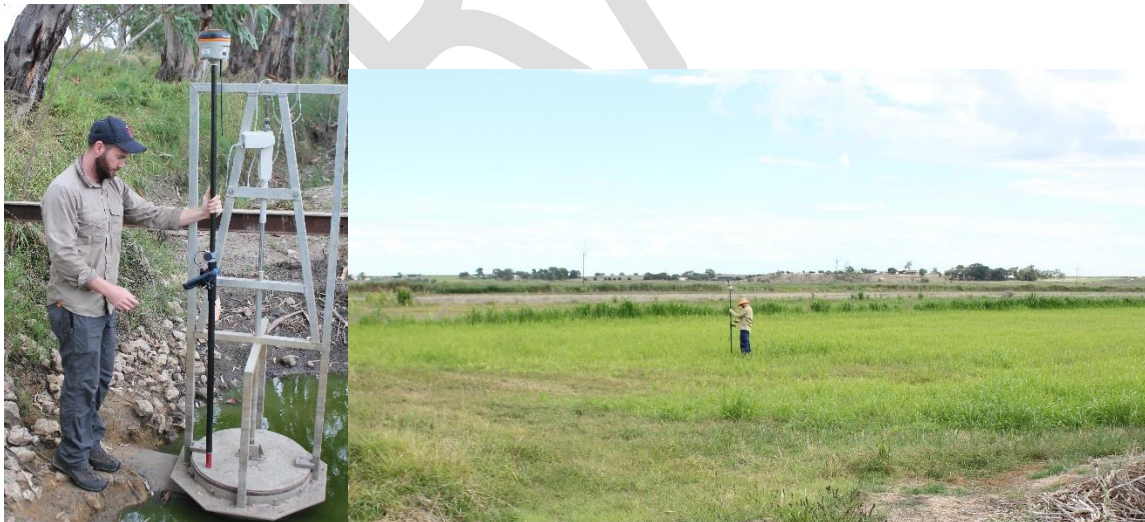
Figure 2. DGPS surveys undertaken by DEWNR staff to obtain the heights of irrigation infrastructure outlets (left) and the natural land height within irrigation bays (right).
