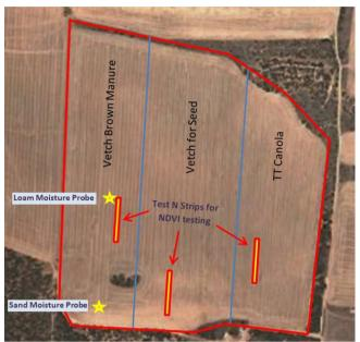
NDVI Trial paddock showing initial 2015 test strips and 2013 break crop treatments. One Nitrogen test strip was included for each break crop treatment
