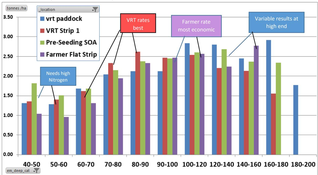
Example where the previous EM38 unit comparison graph has led to zone and rate refinement.
