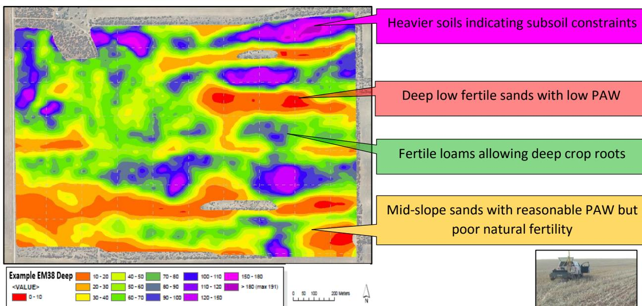
2. These EM38 maps are used to target 5 key soil testing areas to ground test the map information. The deep soil testing is done at 4 depths to 80cm, and analysed for texture, fertility, moisture content and subsoil constraints.
