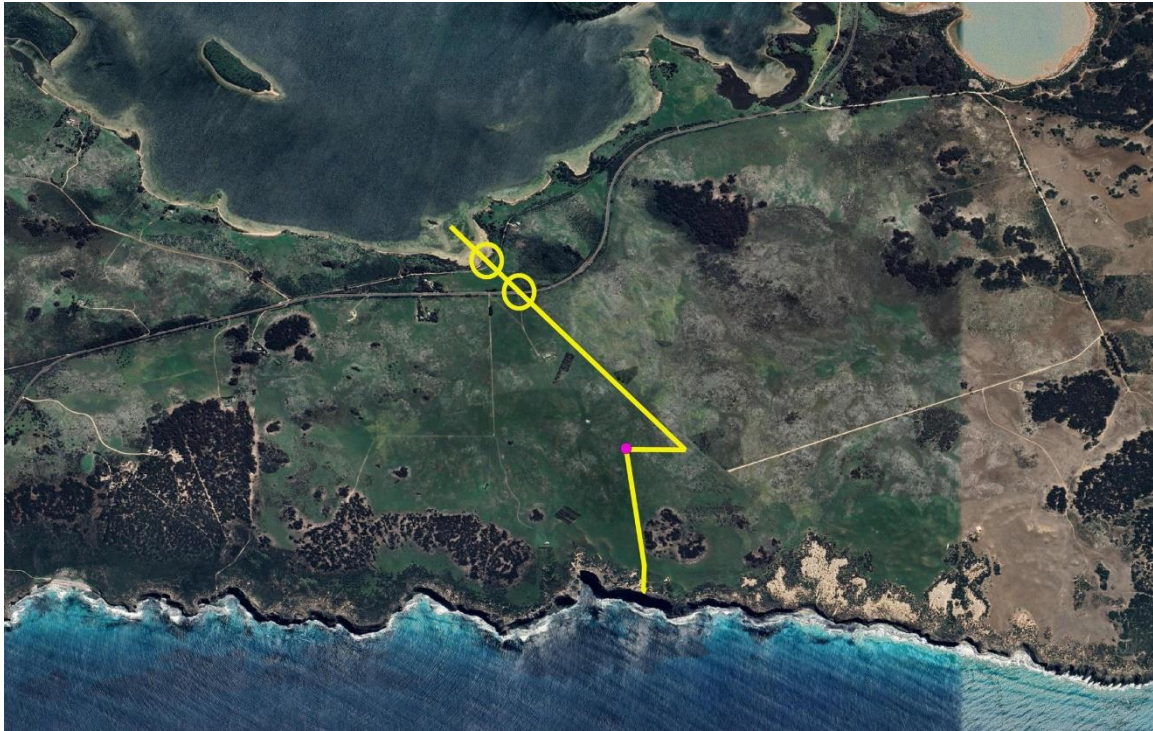
Figure 5. Alignment of the cat barrier fence across the isthmus connecting Dudley Peninsula to the western section of the island. To the south the fence terminates on a cliff and to the north the fence will run into Pelican Lagoon beyond the low tide mark. Two gaps in the fence are denoted by yellow circles.
