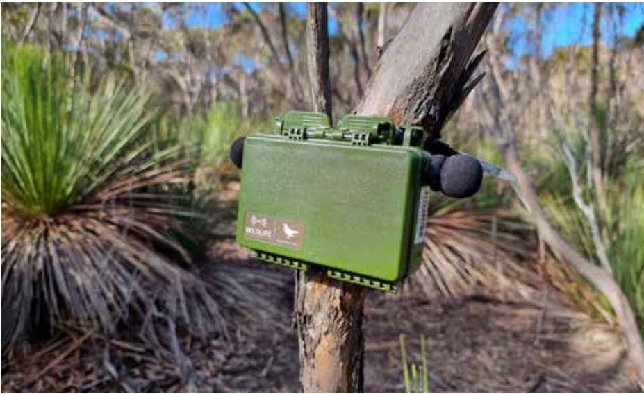
Image right: A bioacoustic recorder capturing the sounds of fauna in revegetated and remnant KI Narrow-leaved Mallee Woodland.
