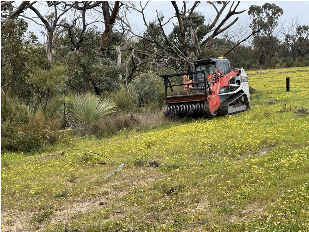
Figure 2. Forestry Mulcher (Correll) - Takeuchi High Flow Track Loader with Fecon Mulcher attachment operating at site L34a.
