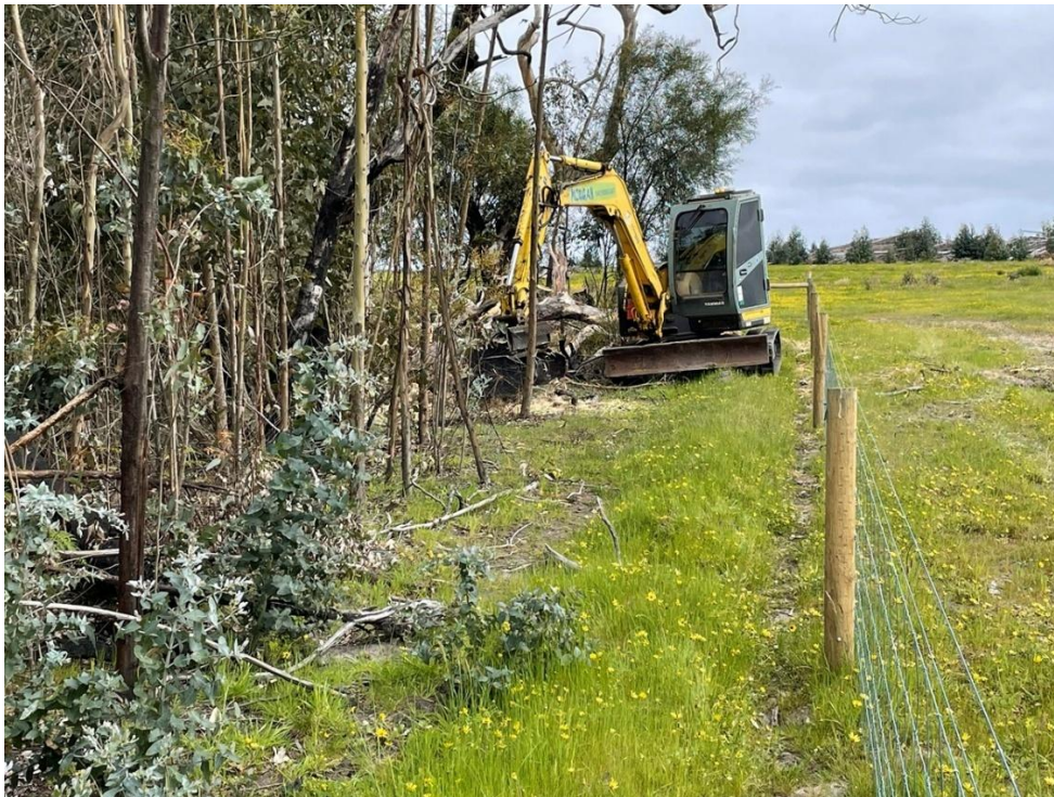
Figure 5. Flail Mower (Morgan) - Yanmar excavator with a Flail Mower head operating at site H5
