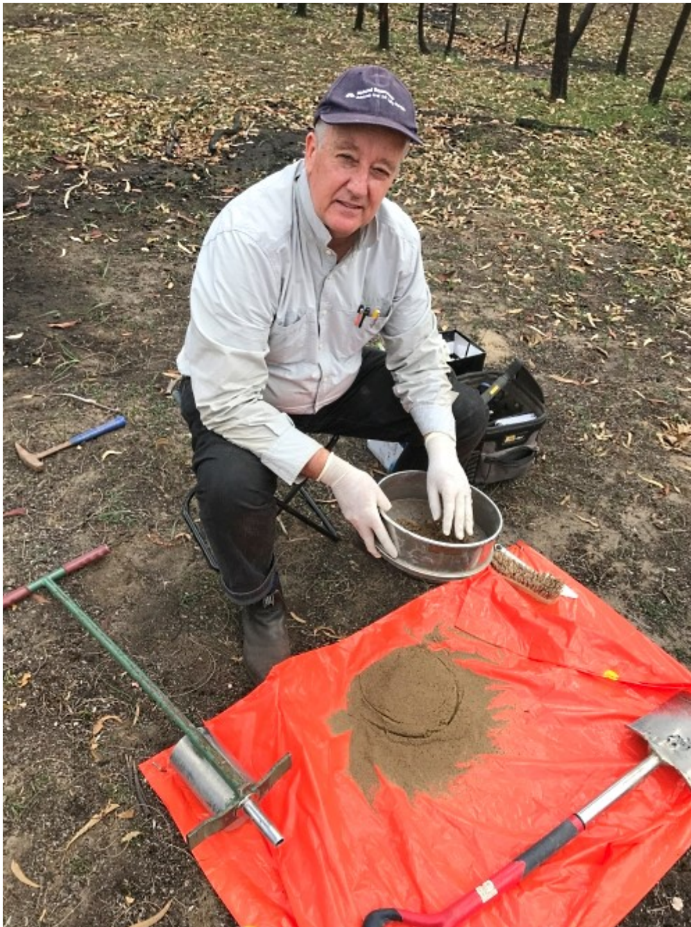
Project manager James Hall preparing soil samples using sterile techniques for soil DNA analysis.
