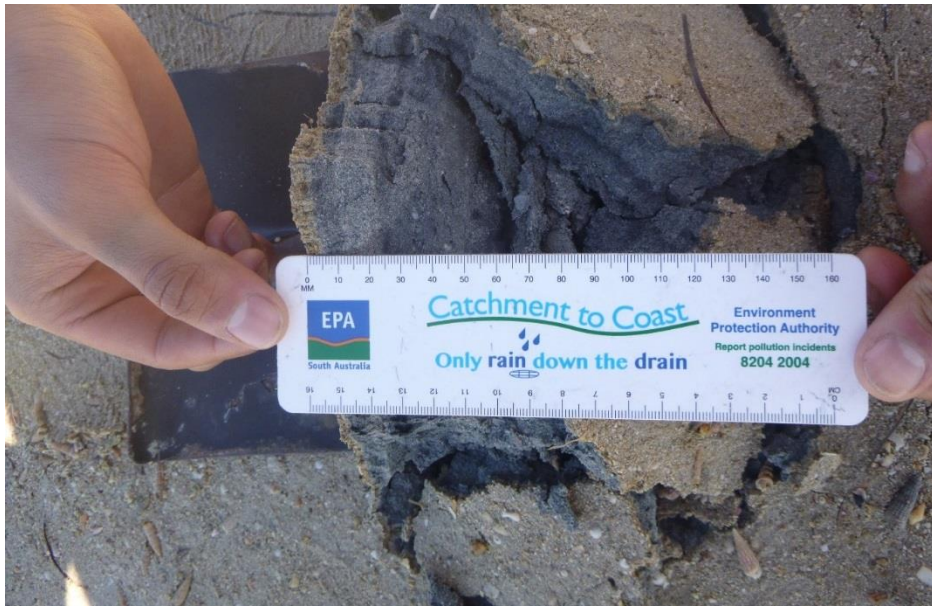
Figure 1: Photograph of benthic sediment top layer removed for assessment of anoxic layer and, presence and depth of burrows.
