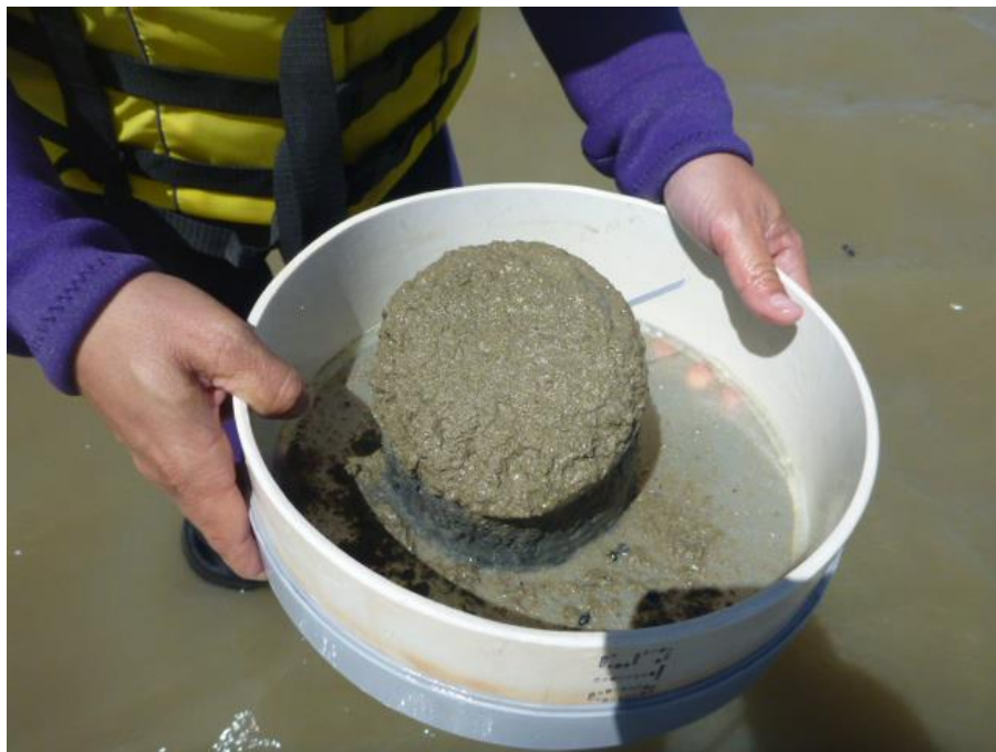
Figure 4: Remaining cored sediment section on sieve after it has been removed from PVC corer.
