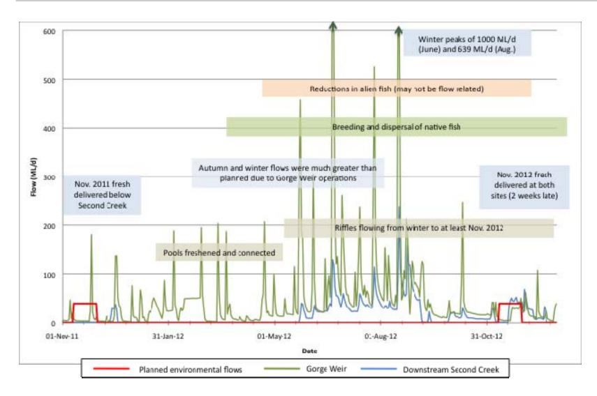
Figure 11: River Torrens – Gorge Weir to Torrens Lake trial reach hydrology, as measured at the weir and below the Second Creek junction, showing key flow \_\_\_\_\_events and environmental outcomes for Year 1, November 2011 to December 2012
