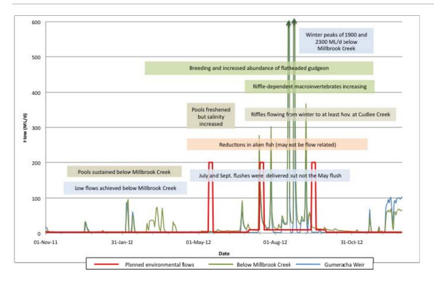
Figure 10: River Torrens – Gumeracha Weir to Kangaroo Creek Reservoir trial reach hydrology, as measured at the weir and below the Millbrook Creek junction, showing key flow events and environmental outcomes for Year 1, November 2011 to December 2012
