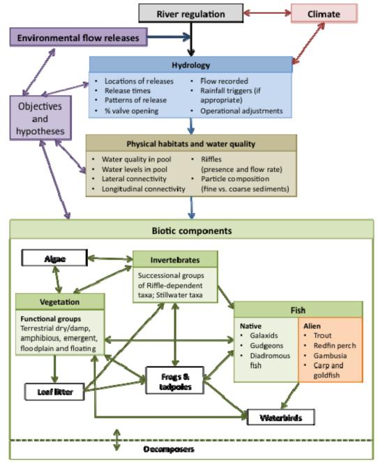
Figure 6: Conceptual model of the logic and environmental indicators used for monitoring the environmental flows trial
