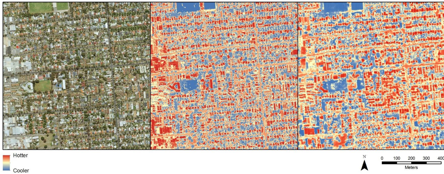
Figure 6: Mitcam case study area showing aerial photography (left) alongside heat mapping from LST modelling (centre) and airborne thermal imagery (right)
