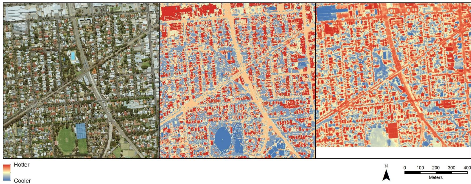
Figure 7: Unley case study area showing aerial photography (left) alongside heat mapping from LST modelling (centre) and airborne thermal imagery (right)
