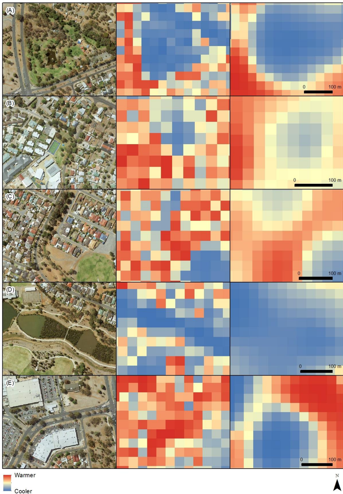
Figure 17: Examples from the Elizabeth and Andrews Farm case study areas showing aerial photography (left) alongside heat mapping from LST modelling (centre) and Landsat thermal imagery (right)
