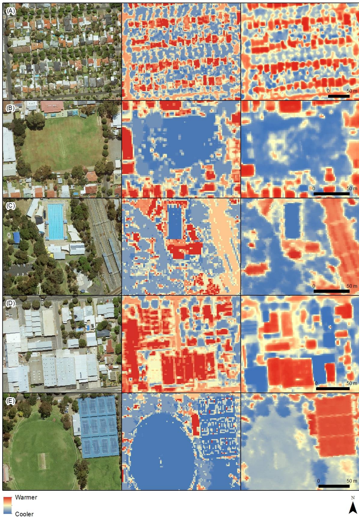
Figure 11: Examples from the Mitcham and Unley case study areas showing aerial photography (left) alongside heat mapping from LST modelling (centre) and airborne thermal imagery (right)
