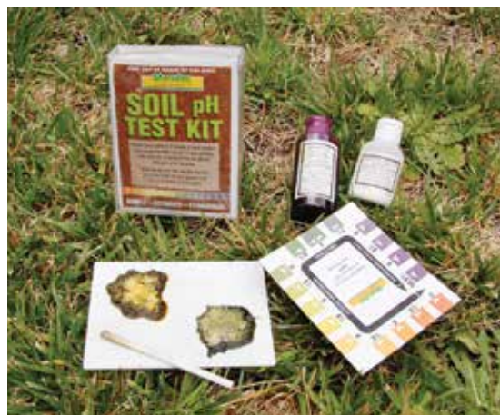
Figure 52. Field pH testing kit
