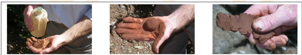
Figure 1. Hand texturing soil samples in the field
