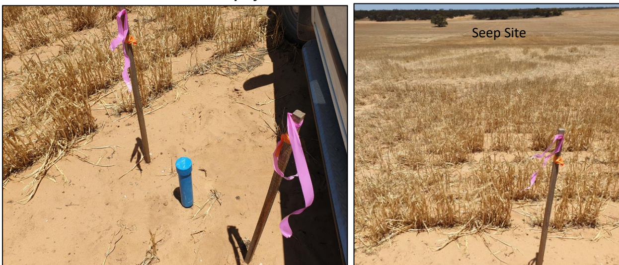
Photo 10. Soil Moisture Probe on top of Sandhill
