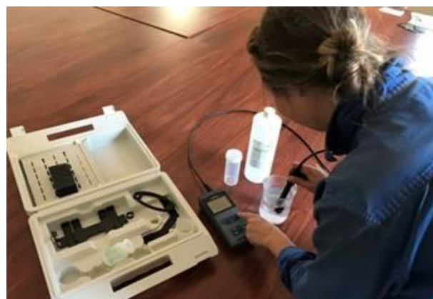
Photo 4: Landscape officer conducting water salinity testing with new salinity meter
