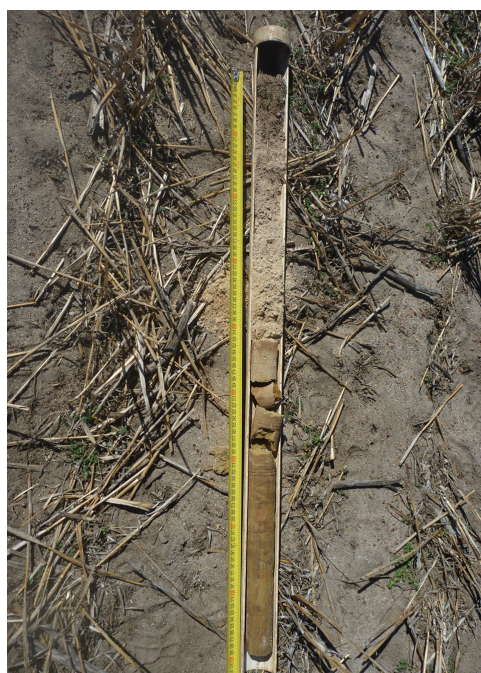
Figure 6. Low production coarse sand on poor structured clay.
