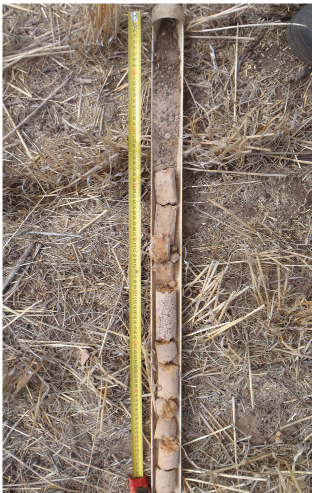
Figure 1. Low production shallow sand on poorly structured clay
