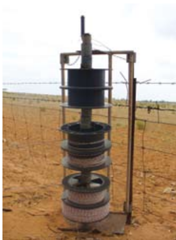
Device made for reeling up braided wire. One reel can be wound up at a time due to a locking mechanism.
