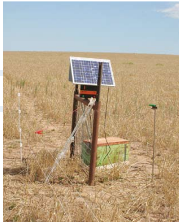
Solar energiser system in standing barley crop.
