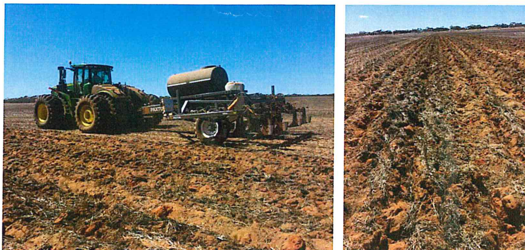
Figure 4. BigFIG 'Paxton' plough deep ripper with inclusion plates and liquids cart
