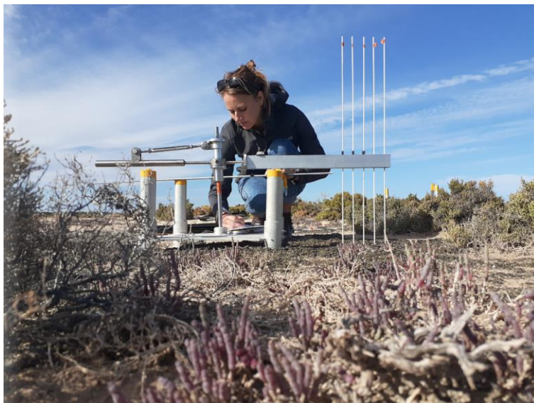
Photo 12: Sediment Elevation Table monitoring being carried out by Landscape Officer at Cowleds Landing (Eight-Mile Creek). Data collected will contribute to a report by Adelaide University on blue carbon stocks, comparing this site to other sites in our region and other regions of South Australia
