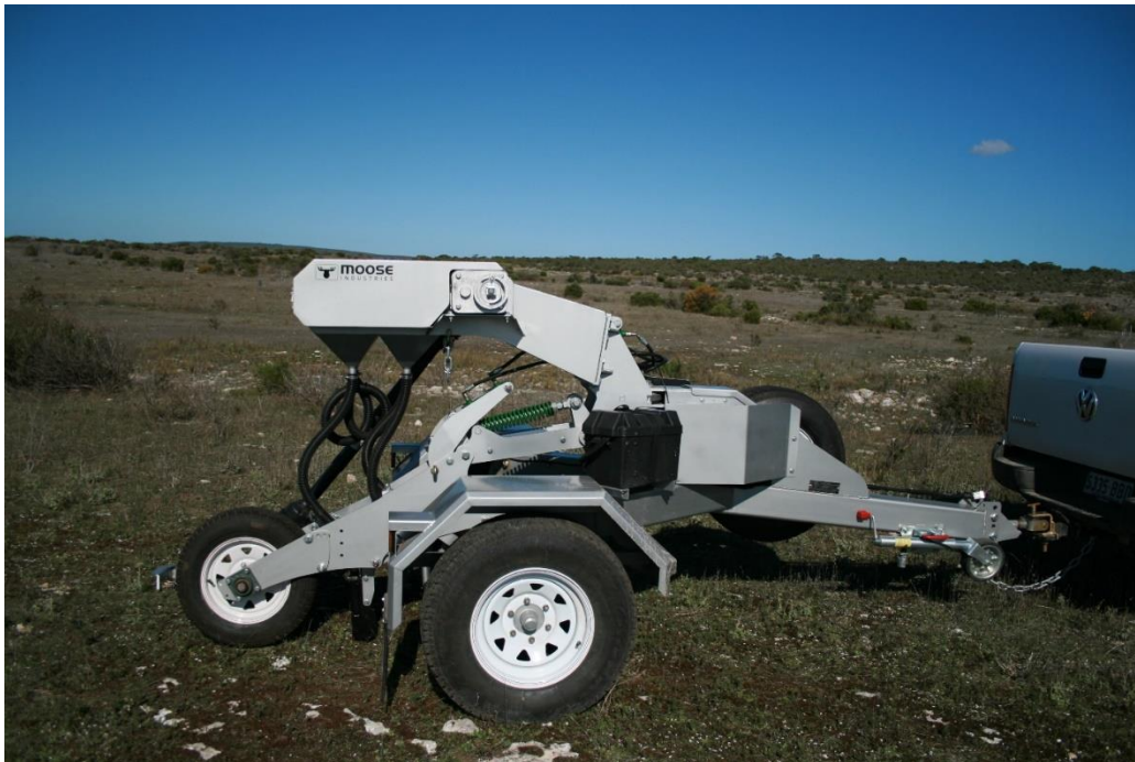
Photo 3: The new direct seeding machine designed and built in 2014
