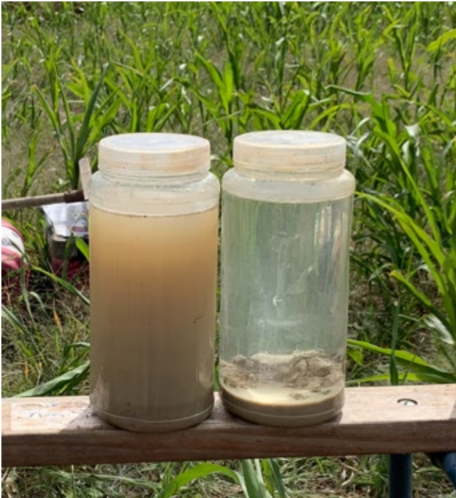
Figure 23: Example of the gypsum jar test. Jar on the left is dispersive soil without gypsum, jar on the right is the dispersive soil with gypsum. The application of gypsum aggregates the clay particles out of suspension. Photo: Edward Scott
