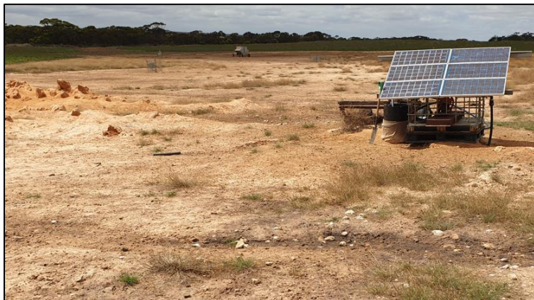
Photo 12. Scald at Dec 2021 with solar pump over sump well and some puccinellia establishing.
