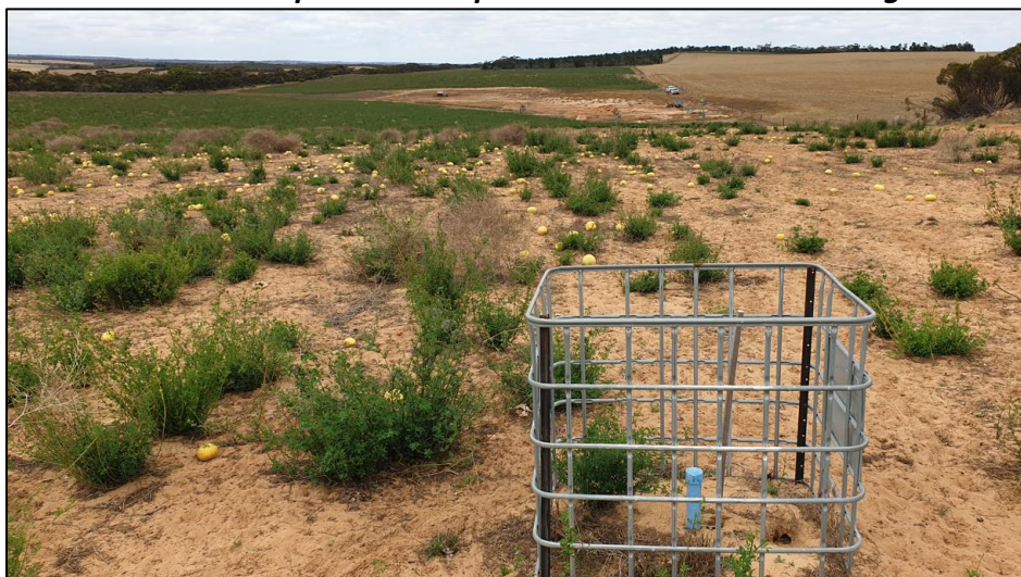
Photo 13. Moisture probe in deep sand above AB Site 2 with good lucerne establishment.
