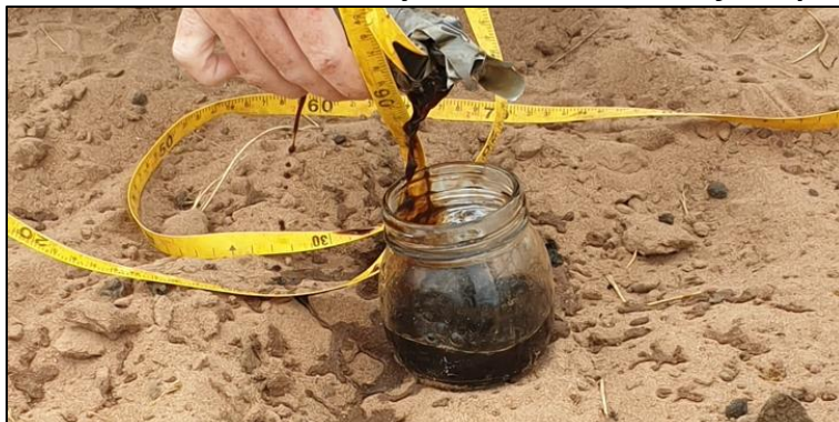
Photo 14. Black, moderately saline water drawn from piezometer 80m southwest of sump.
