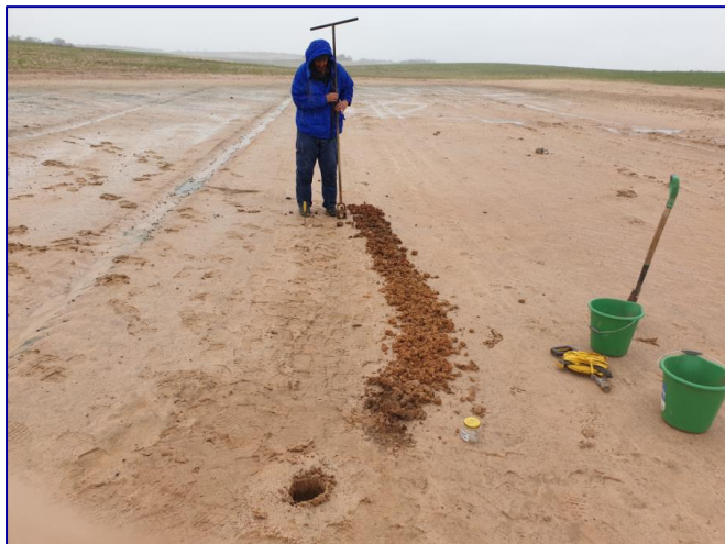
Photo 17. Deep test hole revealing no sloppy clay layer at depth, Seep 3a.
