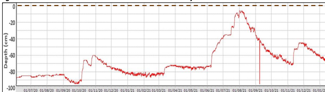
Figure 16. Perched water table level at Site 3b scald July 2020 – Jan 2022
