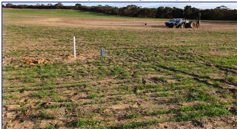
Photo 18. Jericho Seep 3b showing mid-slope piezometer and moisture probe in foreground.
