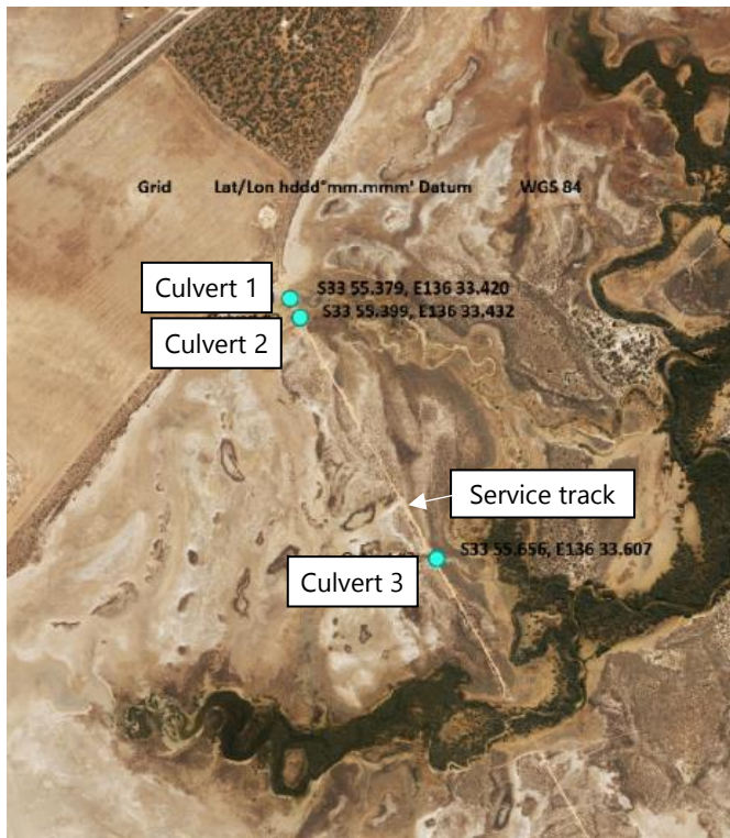
Figure 1: Arno Bay - a third culvert has been installed under an SA Power Networks service track completing the work of restoring tidal flows to saltmarsh
