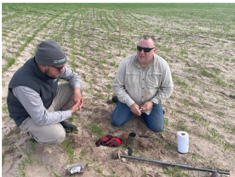
Photo 1: Landscape officer with PIRSA Soil and Land Management Consultant taking a soil bulk density measurement at a soil amelioration demonstration site
