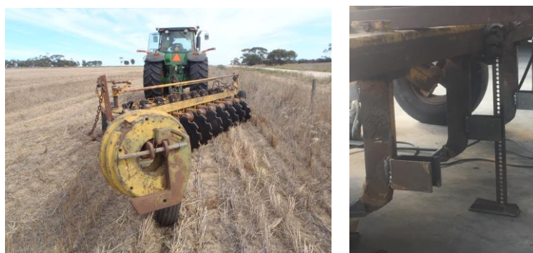
Figure 5. Modified one way disc plough for deep soil mixing.
