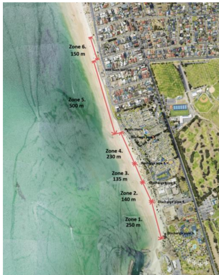
Figure 4-1 Delineation of the nourishment zones along West Beach for the 2021/2022 nourishment campaign.
