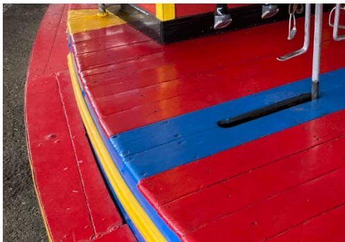
Oregon platform, showing slot allowing horse rods to swing outwards with centripetal motion.
