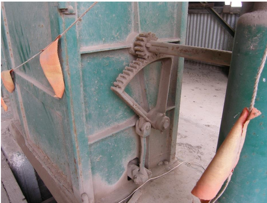
Weighbridge, Islington Railway Workshops. Note the triangular sprockets.
