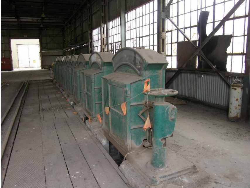
Weighbridge, Islington Railway Workshops
