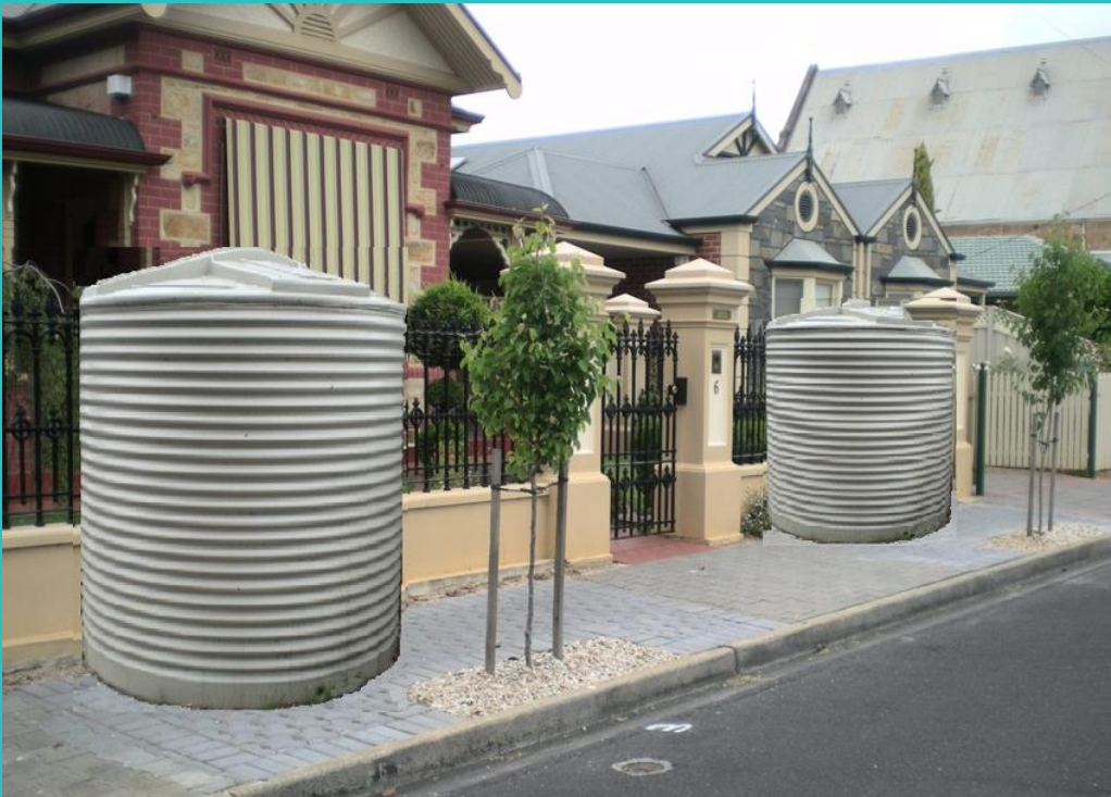
Above image: The rainwater tanks represent the annual amount of water (4000 litres) delivered to the soil through 8m 2 of permeable pavement. Photograph taken 29 October 2010 (39).
