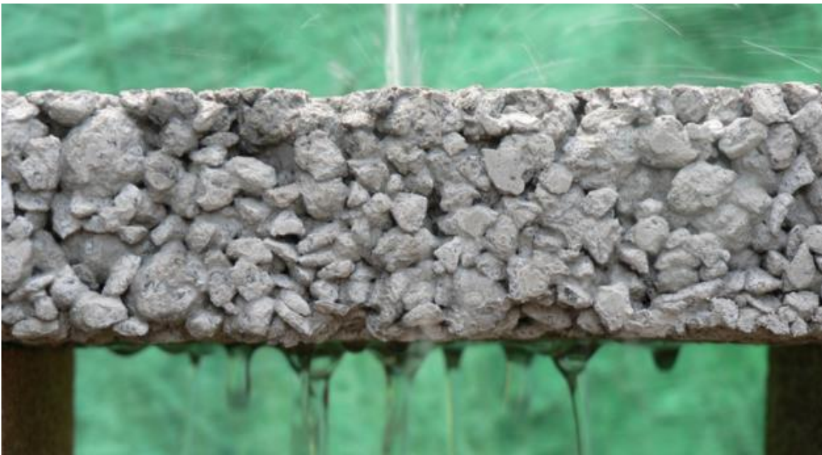
Figure 3. Permeable pavement has been used to great effect in both residential roads and foot paths within the City of Mitcham (Photo: TecEco, 2020 (67)).
