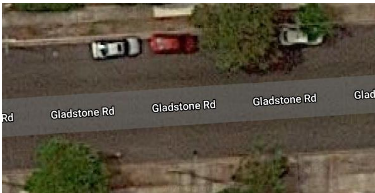
Figure 2. A typical footpath, street verge, road, gutter and water table area only contain approximately 15% permeable surfaces (40)
