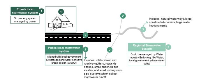
Considering the elements of the stormwater system separately provides an opportunity to clearly articulate where responsibility sits for each element of the system. Appropriate legislative frameworks, governance arrangements and funding mechanisms can then be developed for each element.
