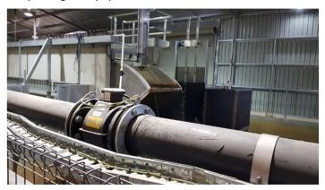
The picture above is from Rubicon's hydraulics laboratory, where its metering systems are extensively tested and calibrated.
