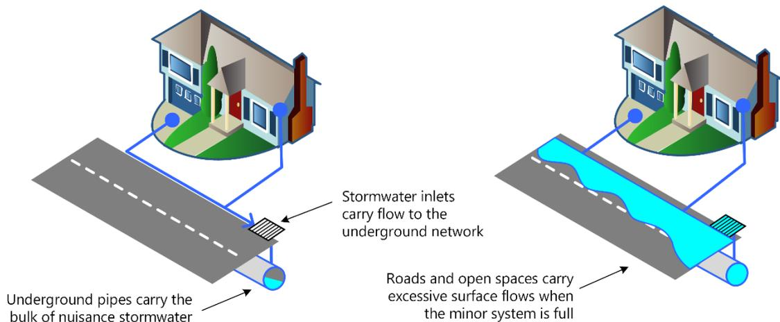
The ‘**minor system**’ – typically underground pipe networks and other infrastructure to collect and convey urban runoff during most small rainfall events (these being the bulk of all rainfall events). If, however, runoff exceeds the minor system’s capacity then surface flow occurs.
