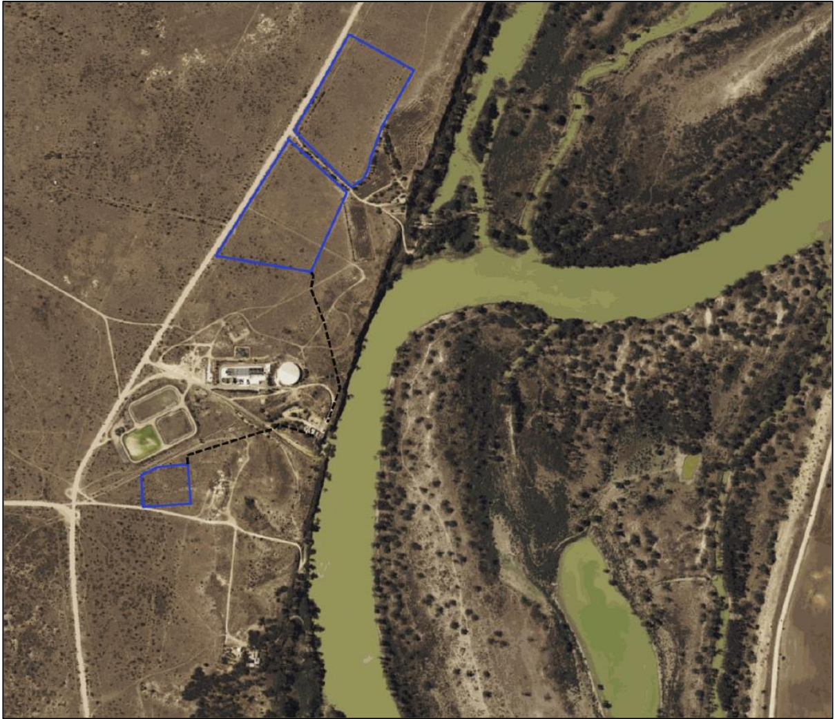
Figure 3: Shows the solar array areas (blue outline) and associated electrical cable routes (dashed black line). Note that the cable route is proposed to be above ground (overhead) in the northern half and underground in the southern half.
