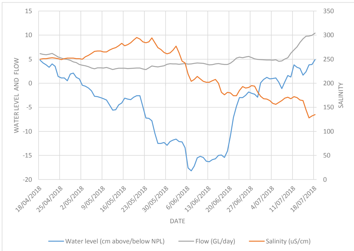
Figure 12. Lock 6 Weir pool lowering - winter 2018
