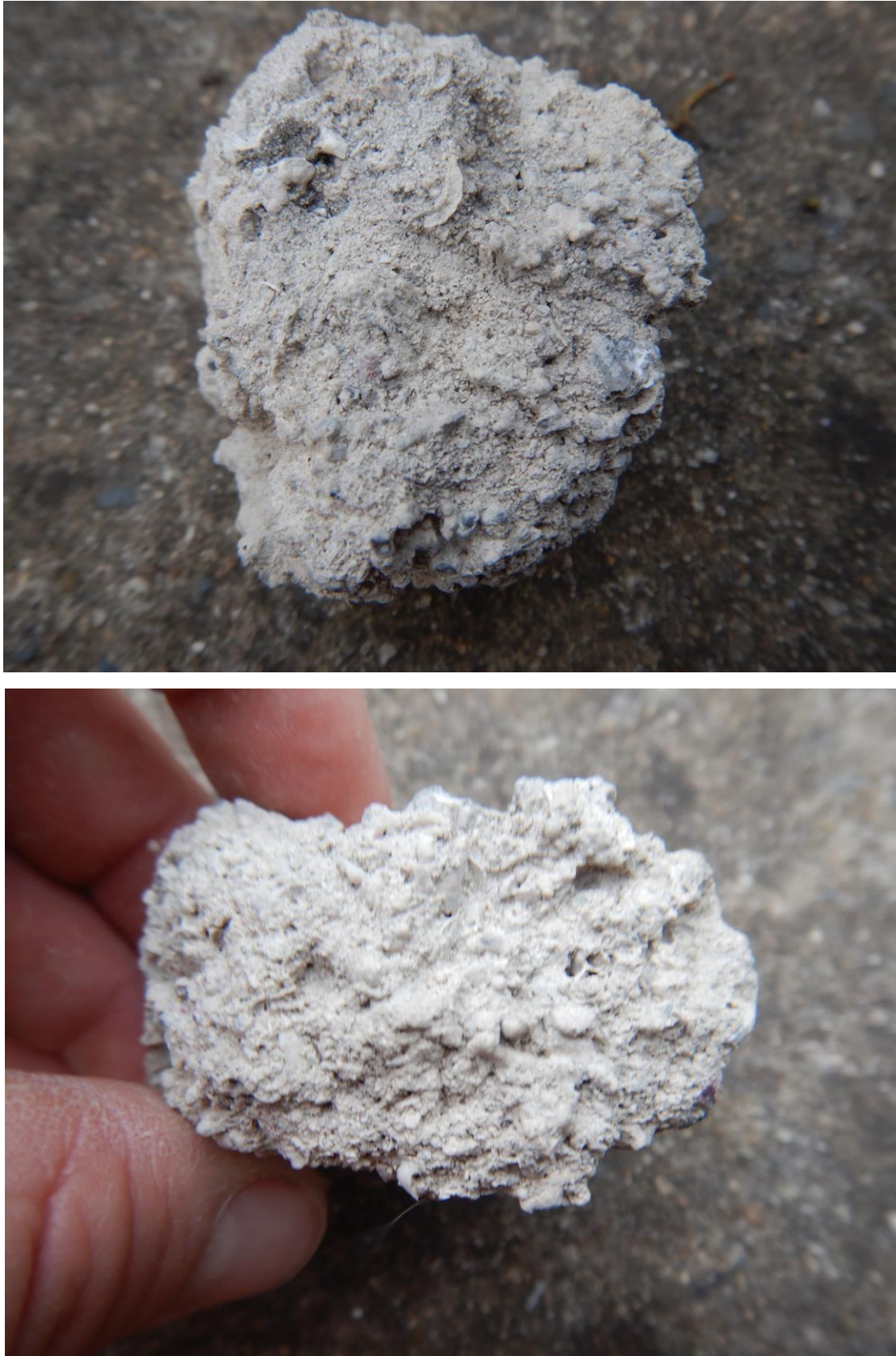
Figure 8. Calcrete cut through by OEM Vibecore from previous project (not Pt Stanvac area) shows cutting potential of Vibecore unit. (A disc shape until chiselled out of the end of the core).
