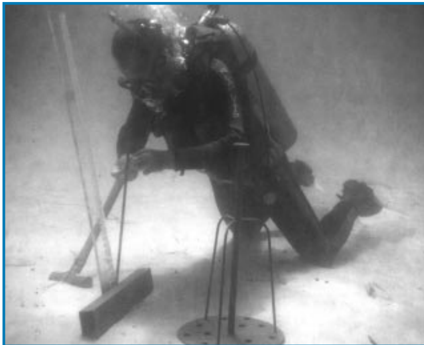
Figure 8 Diver measuring sand level rod.
