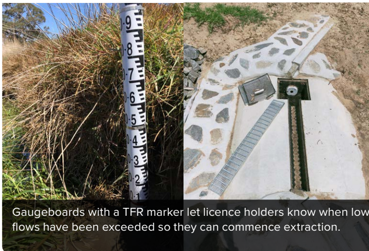
End caps have an orifice cut into them that corresponds specifically to the TFR for individual sites.
