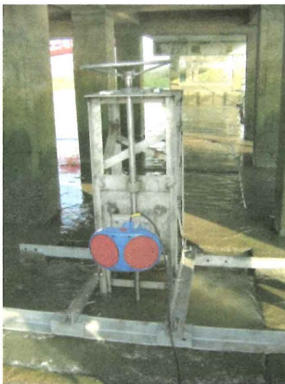
Figure 3 A 300 kHz H-ADCP at Songpu Bridge hydrology station in Huangpu River, Shanghai, China
