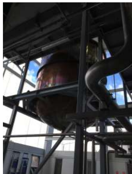
Copper kettle, showing riveting and rounded base. Source: DEW Files 24 March 2021.
