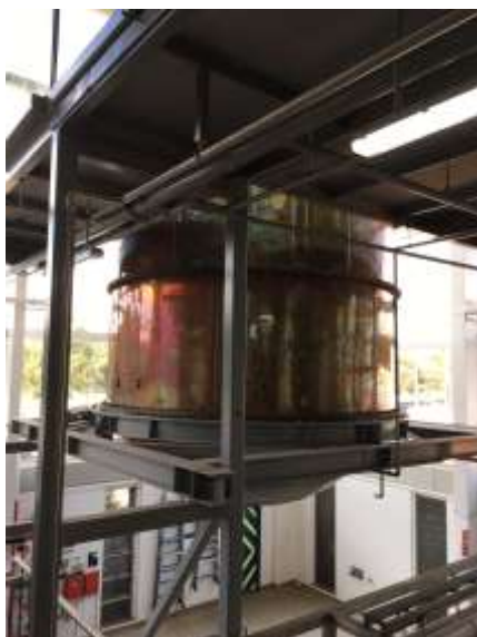
Copper kettle, showing riveting and rounded base. Source: DEW Files 24 March 2021.
