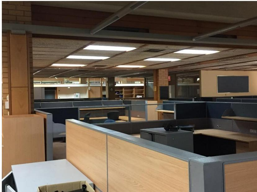
View of office space in the Salisbury Civic Centre view from 1981 addition to 1975 building, note the dropped ceiling in the transition between the two spaces.
