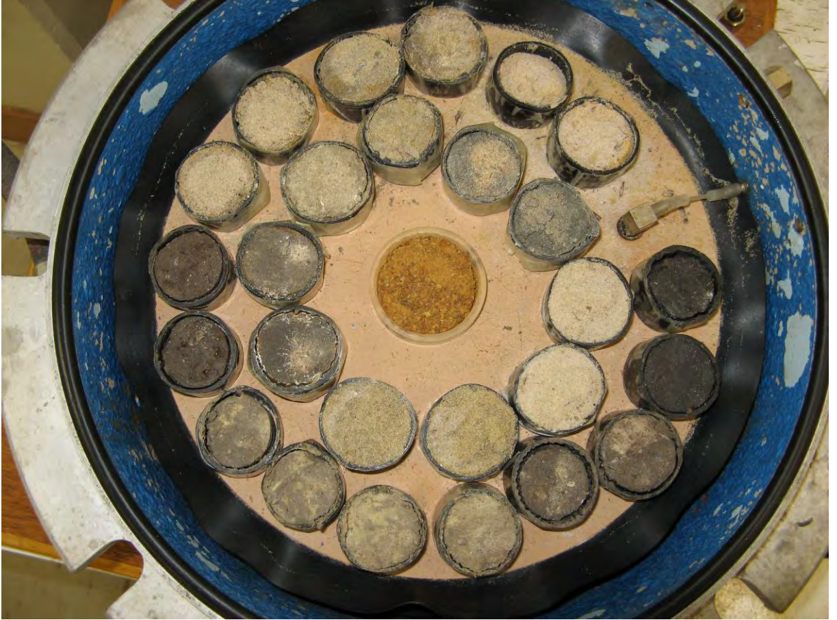
Figure 15. Pressure plate showing sub-samples and heat shrink liner. Some shrinkage can be seen with some of the samples.
