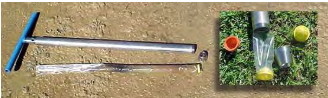
Figure 8. Photograph of sampler, showing auger tube, a sample in liner, sample catcher (yellow plastic), plastic liner for sample and cutting shoe. Image from Dormer Engineering.
