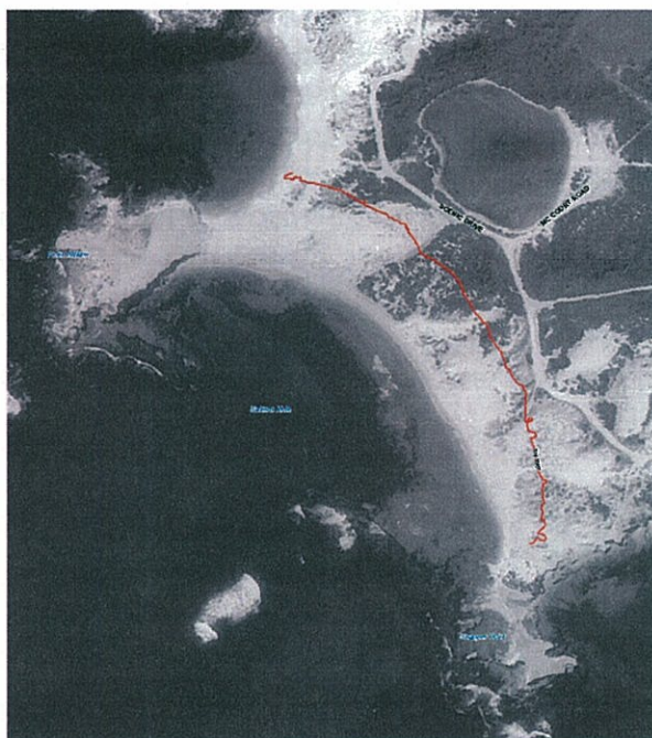
2007 erosion scarp (red line) position on a 1975 aerial photo.
